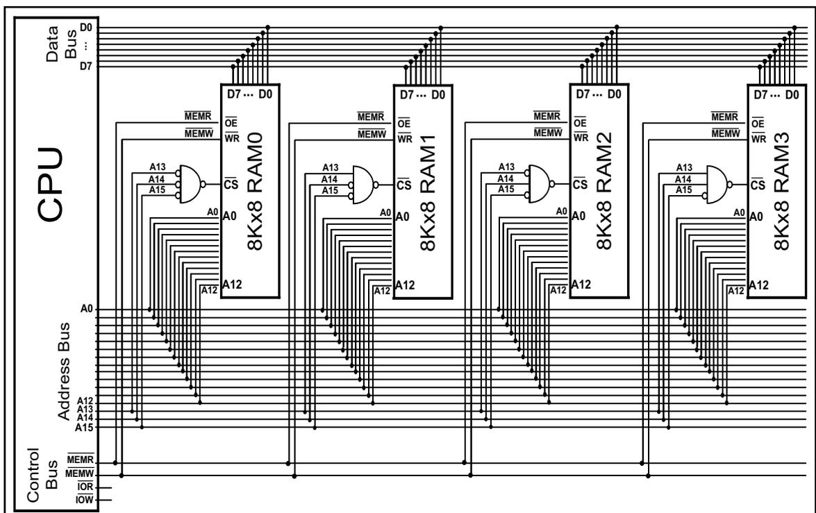
Figure 0-20. Connecting Four Memory Chips to the CPU
