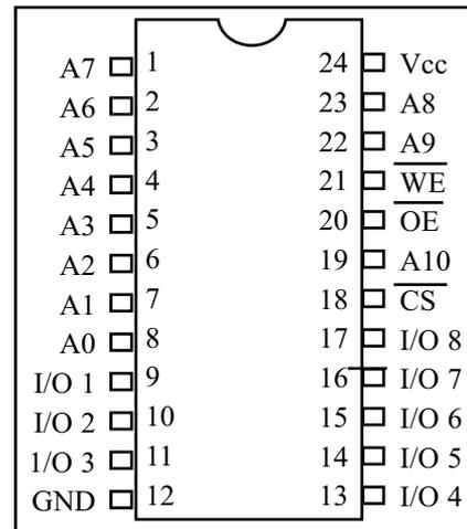
Figure 0-11. 2K × 8 SRAM Pins
