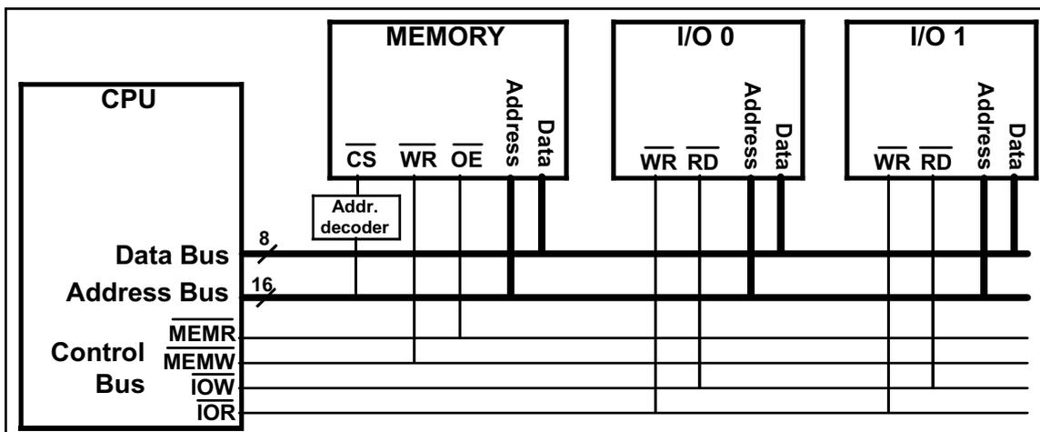
Figure 0-17. A Simple System Using Peripheral I/O
