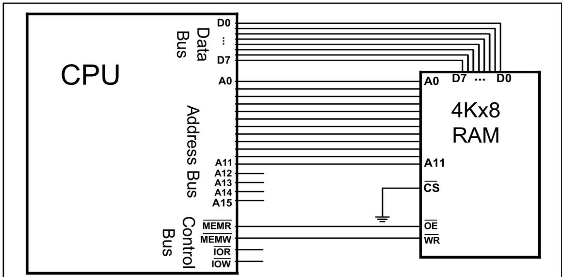
Figure 0-19. Connecting Memory Directly to the CPU
