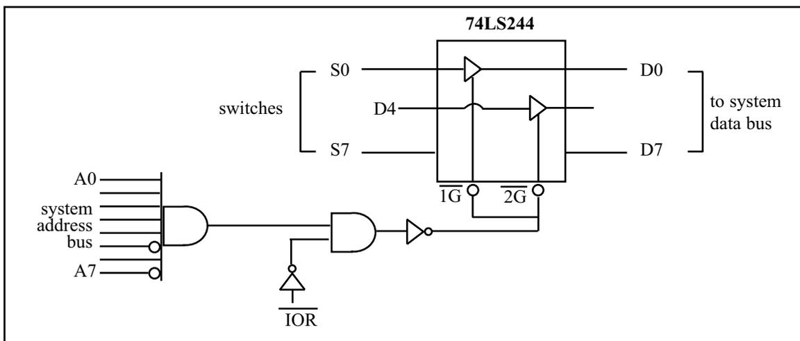
**Figure 0-28. Design for Input Port Address 5FH**
