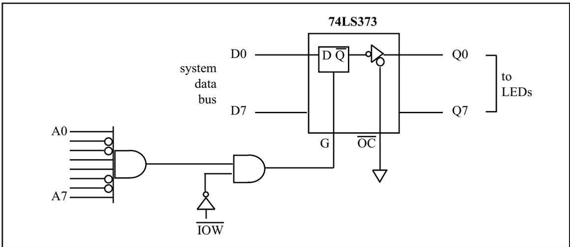
Figure 0-23. Design for Output Port Address 99H.
