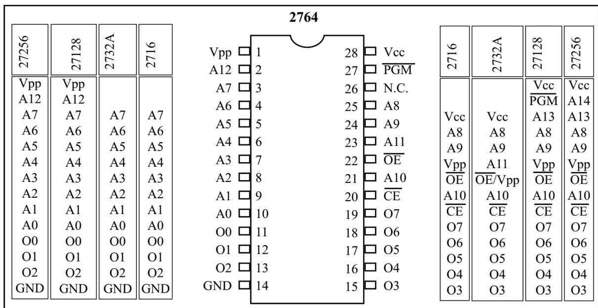
**Figure 0-10. Pin Configurations for 27xx ROM Family**
