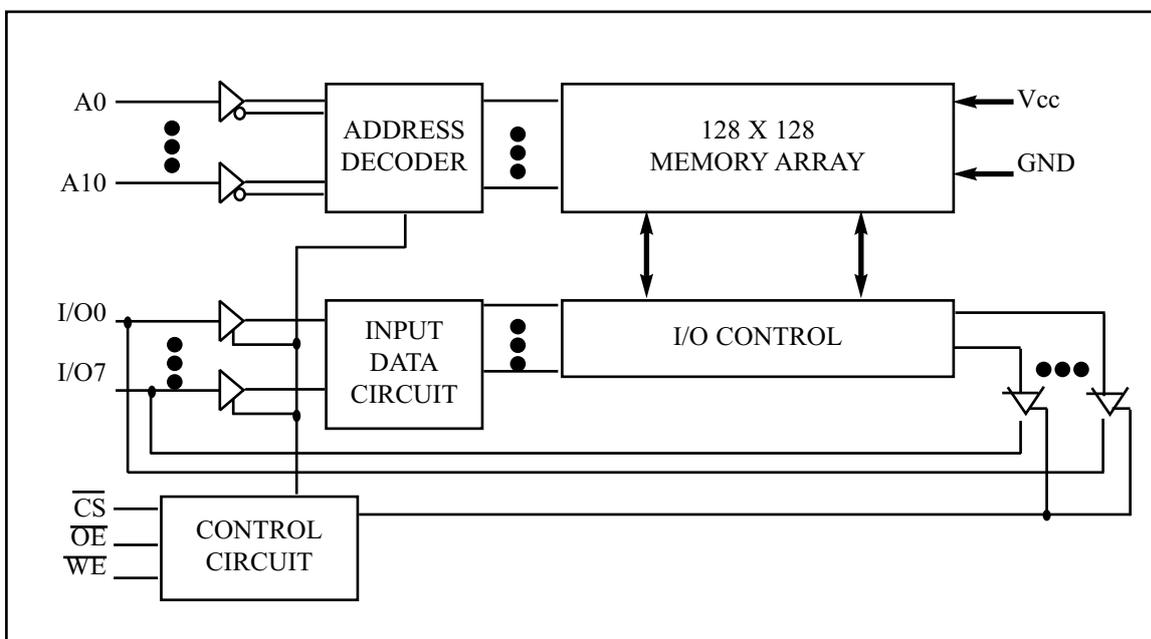
Figure 0-12. Functional Block Diagram for 6116 SRAM
