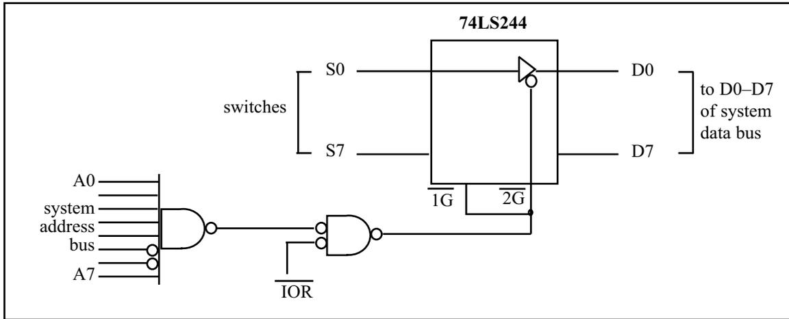
**Figure 0-27. Design for Input Port Address 9FH**
