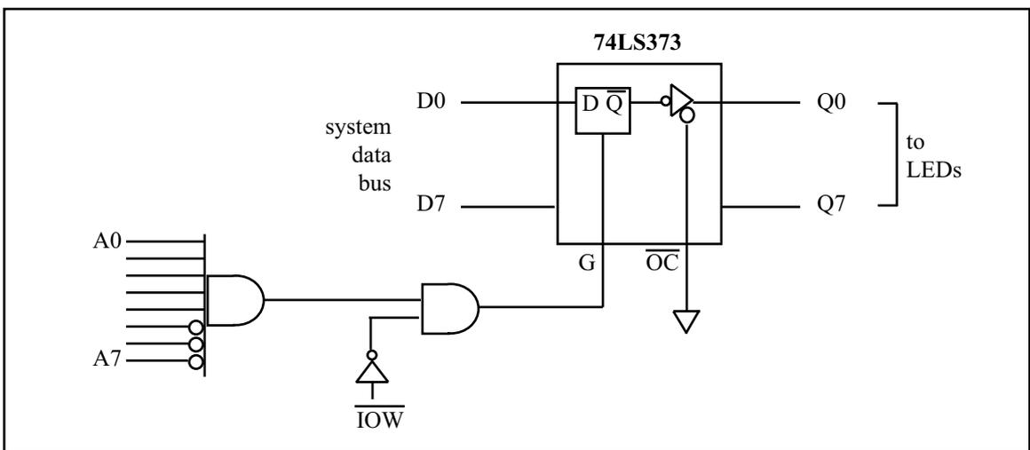
Figure 0-24. Design for Output Port Address 1FH
