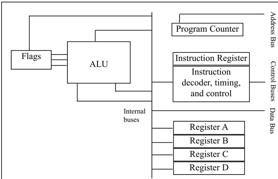
Figure 0-31. Internal Block Diagram of a CPU
