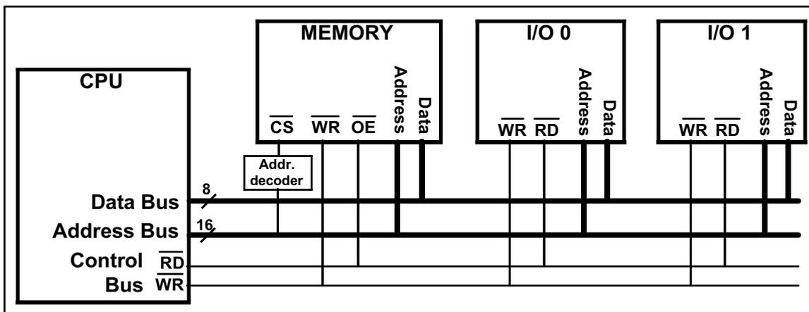
Figure 0-30. A Simple System Using Memory-Mapped I/O
