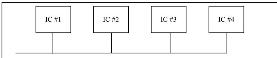
**Figure E-1. Daisy Chain Connection (not recommended for power lines)**
