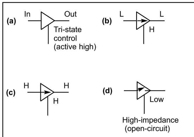
**Figure H-9. Tri-State Buffer**
