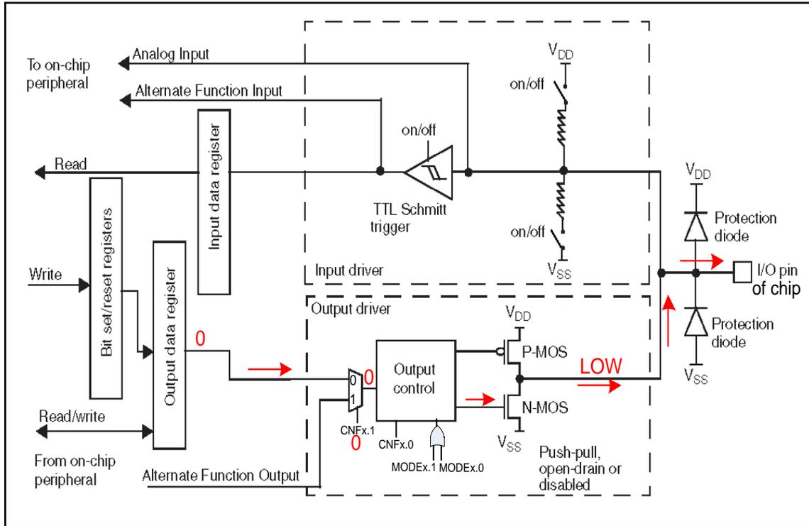
**Figure H-12. Outputting (Writing) 0 to a Pin in the STM32F10x**
