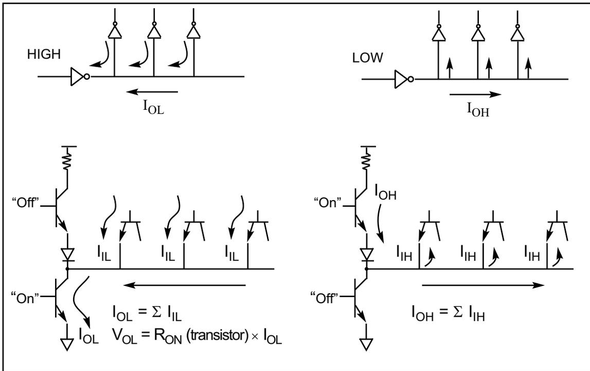
**Figure H-7. Current Sinking and Sourcing in TTL**
