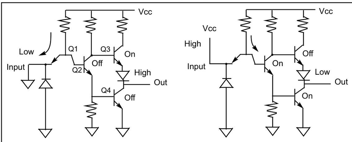
**Figure H-3. TTL Inverter with Totem-Pole Output**
