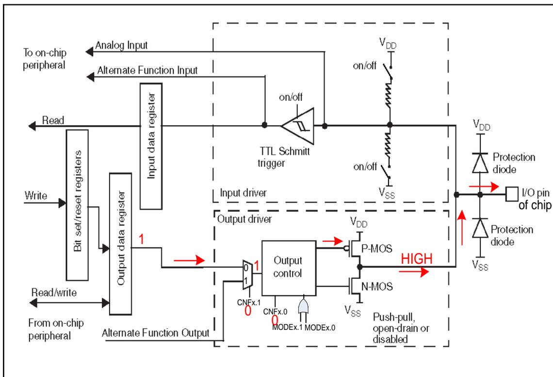
**Figure H-13. Outputting (Writing) 1 to a Pin in the STM32F10x**
