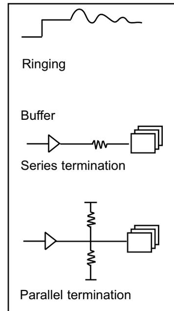
**Figure H-17. Reducing Transmission Line Ringing**
