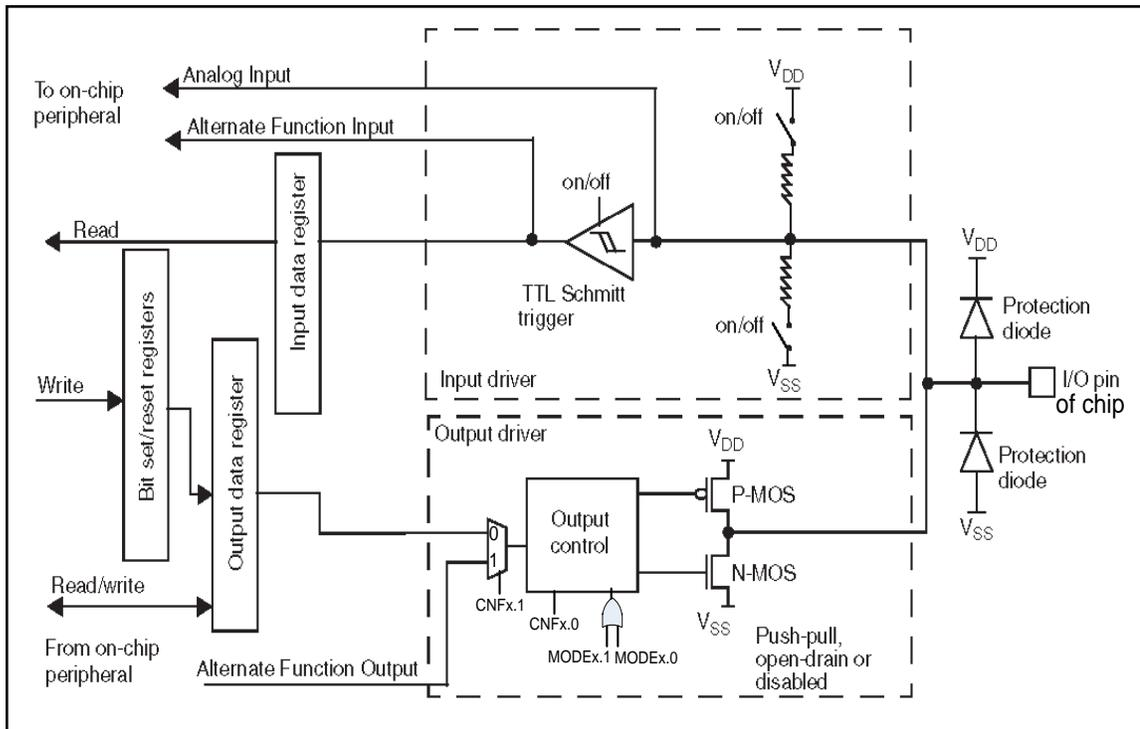
**Figure H-10. The STM32F10x Ports Structure**
