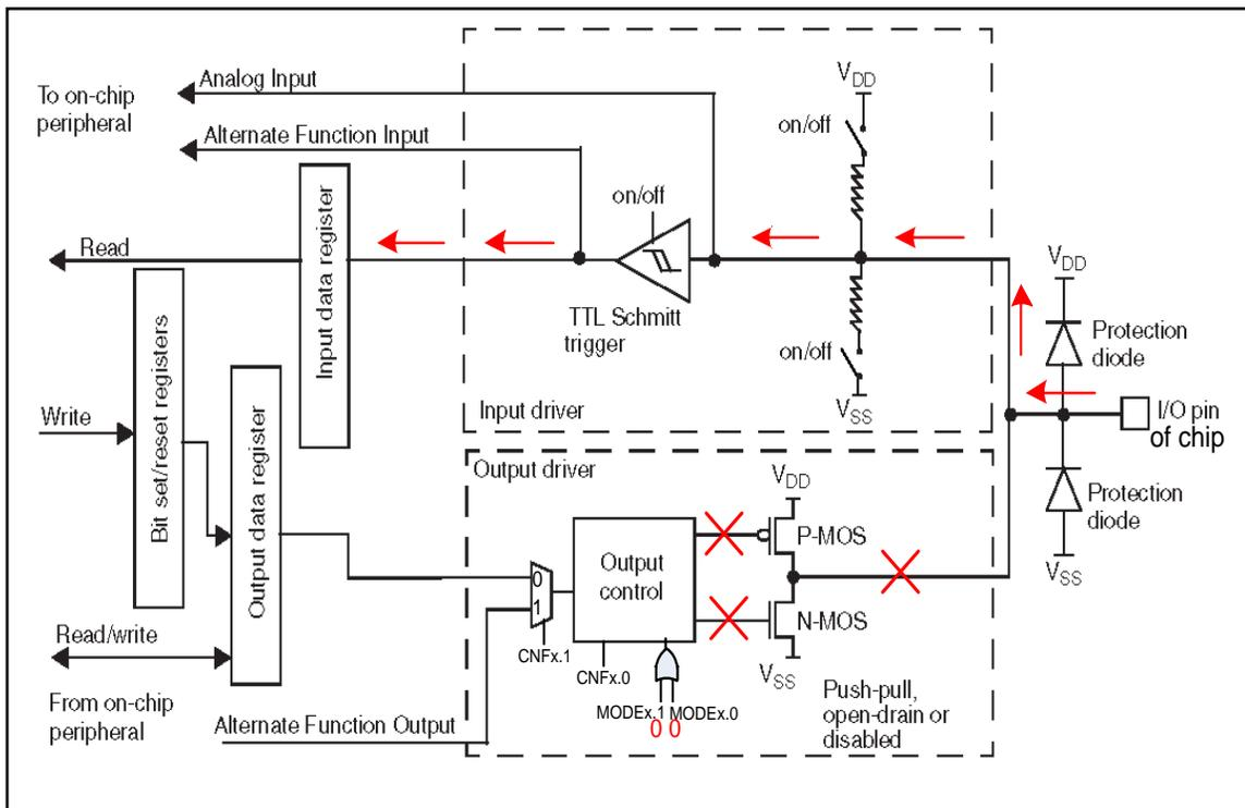
**Figure H-11. Inputting (Reading) from a Pin in the STM32F10x**
