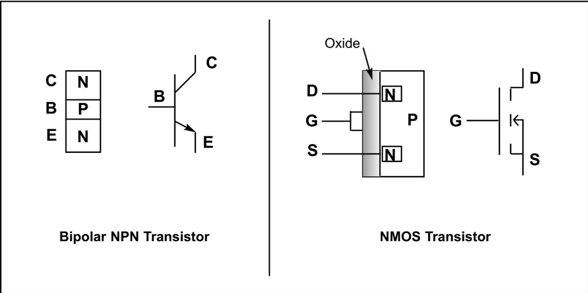
Figure H-1. Bipolar vs. MOS Transistors
