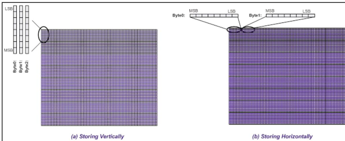
Figure H-7. Storing Data in the LCD Memory of Mono-colored LCDs
