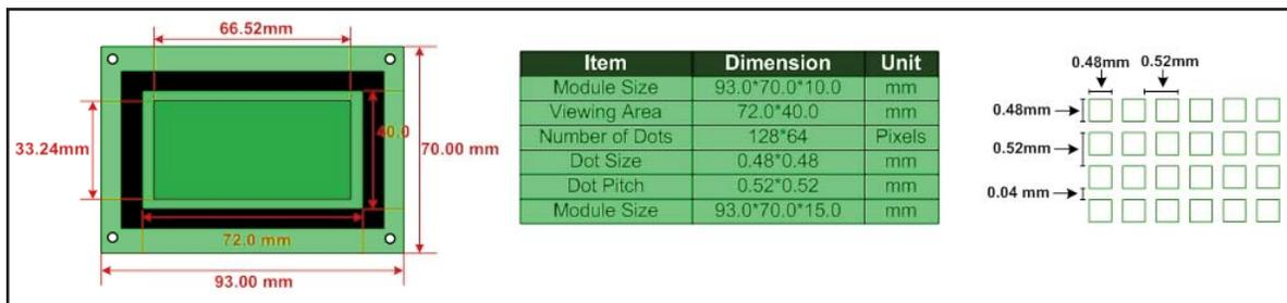
**Figure H-4. Mechanical specifications of a GDM12864 128x64 LCD**
