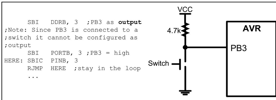
Figure C-14. A Common Mistake, Which Damages I/O Ports
