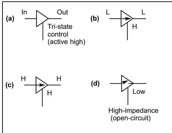
**Figure C-9. Tri-State Buffer**
