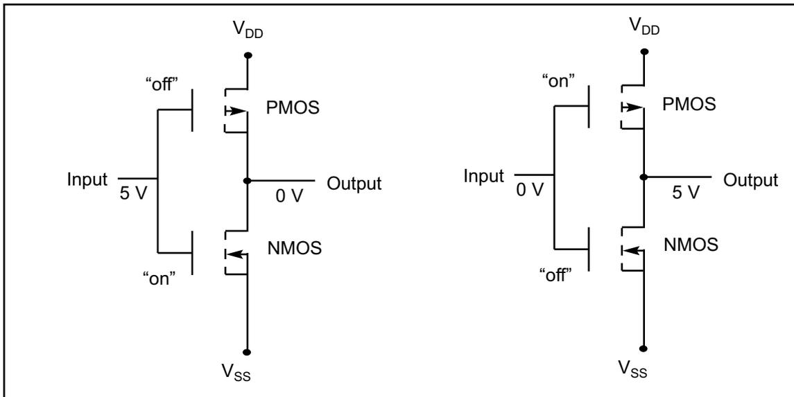
Figure C-4. CMOS Inverter
